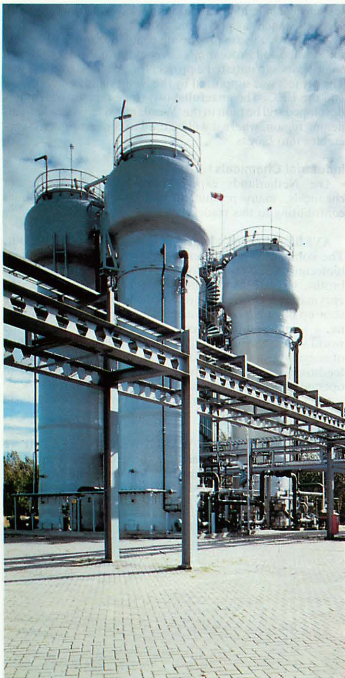
THE UASB REACTOR (Upflow, Anaerobic Sludge Blanket) has been developed through the joint efforts of various universities and the sugar manufacturer, CSM. 42 of these UASB's for industrial waste water treatment have already been installed. Gist-Brocades had assumed all rights to this reactor (foto Gids-Brocades).
