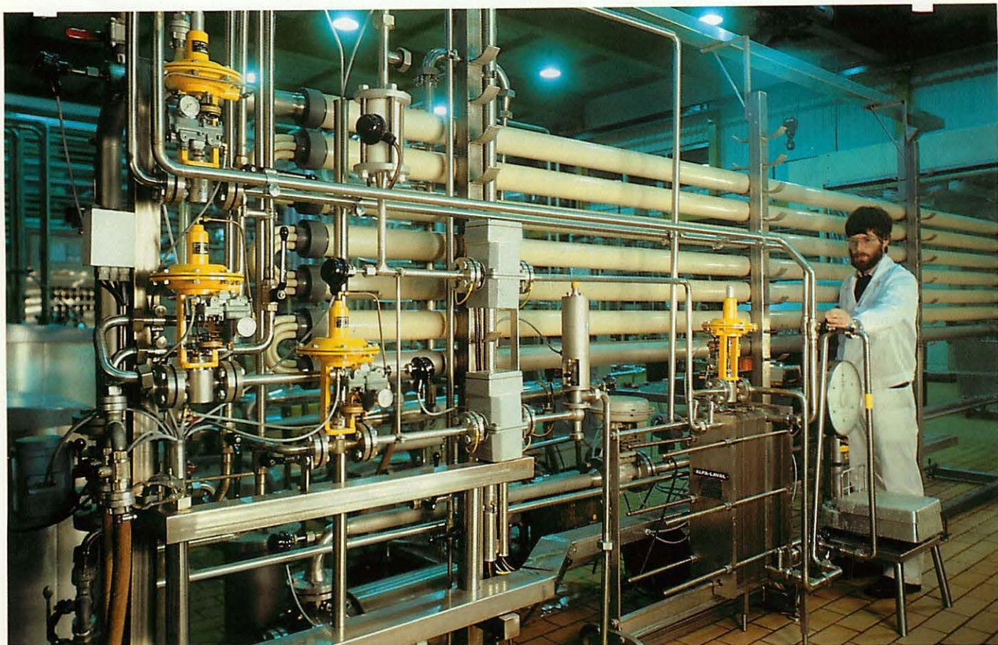
▲ MEMBRANE FILTRATION for dairy products at NIZO (the Netherlands Institute for Dairy Products). The dairy companies support this research institute by contributing a tenth of a cent per litre of milk produced.
