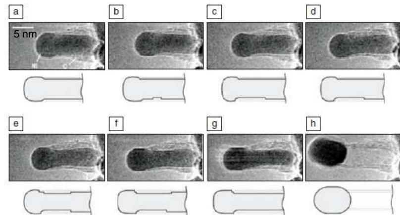
Nikkel catalysts with CH<sub>4</sub>/H<sub>2</sub> @ 2.1 mbar and heated to 536 °C
